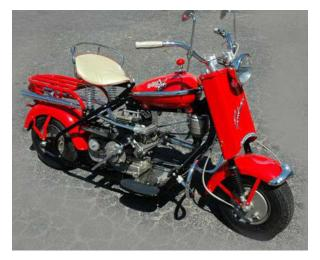
The Cushman was inconvenient at night, since its stator was so weak that it could not supply enough electricity to power the lights.
