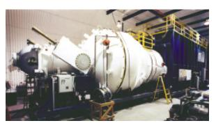
When the beast was fired, an electron beam would cascade down until it hit a target made of tantalum, which would create a very fast, but intense, X-Ray pulse.
